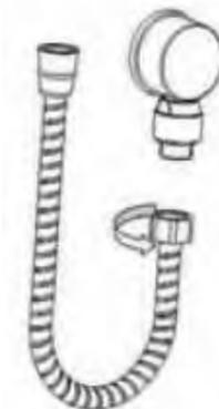
6) Connect the Hand Shower with the Hose as shown in the first page of General Assembly Drawing.
