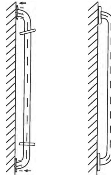
2) Connect the Slide Bar Bracket to the Slide Bar. See detailed photo instructions if needed.
