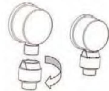
5) Connect the Hose with the Vacuum Breaker as shown in the drawing.
