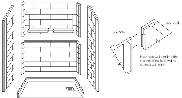
**FEATURES** Dimensional Tolerance  $\pm 1/2"$ . Dimensions needed for site preparation should be measured from the unit. Accessibility Professionals Inc. assumes no responsibility for prep work.
