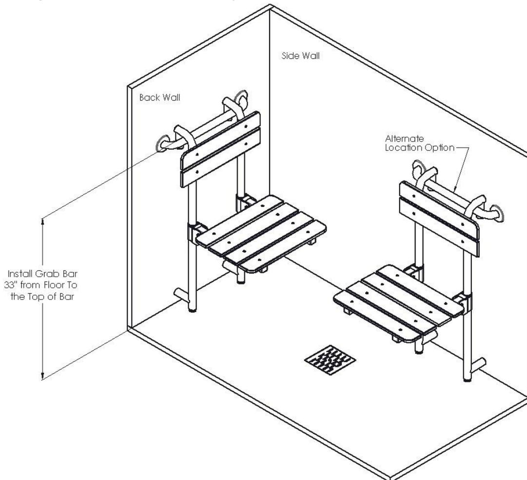
Locate the area in the shower enclosure with 2" solid wood in-wall backing.
