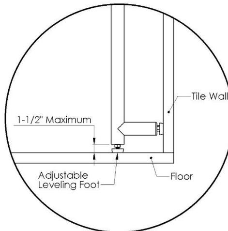
**IT IS EXTREMELY IMPORTANT THE PROFILE SEAT DOES NOT REST EXCLUSIVELY ON THE WALL-MOUNTED GRAB BAR, AND THE TWO (2) FLOOR LEVELING FEET MUST BE SECURE ON A CLEAN, FLAT LOCATION ON THE FLOOR OF THE SHOWER ENCLOSURE FOR PROPER USE.**
