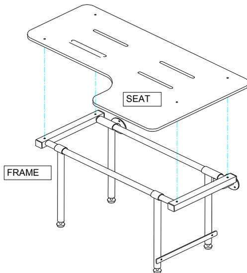
Mount the seat top to the frame in the desired configuration.
