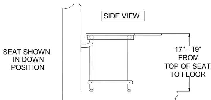
Place the seat in an upright position with the mounting flanges placed firmly against the shower wall.
