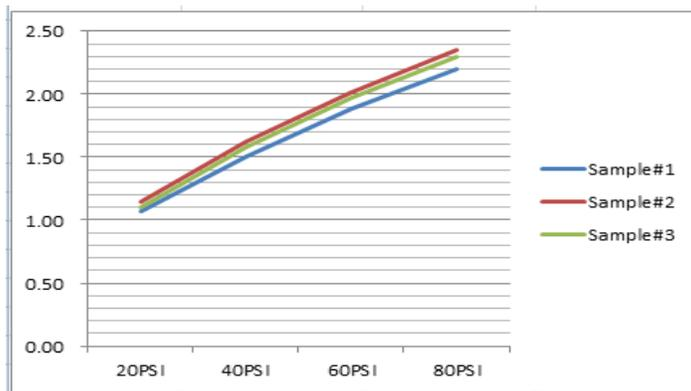
Flow Rate Test Results for Hand Shower with Flow Restrictor
