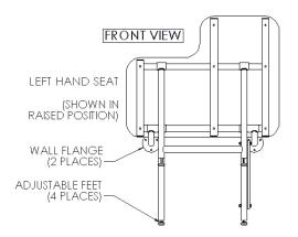
Level the seat by changing the adjustable rubber feet to the desired mounting height (17"-19"). Tighten the lock nuts.
