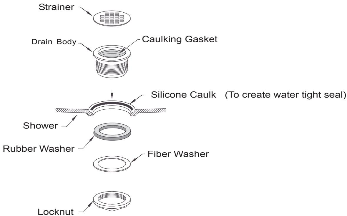
Using a large screwdriver and the tool provided with the drain, tighten the inside caulking nut into the drain body.
